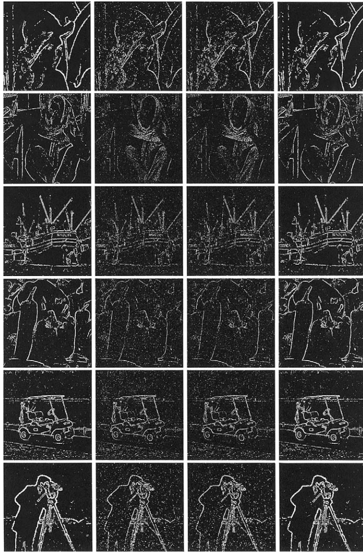
Fig. 8. Edge images of the noisy sample images, column 1–4 are obtained by using, respectively, the DSCANED 1 , the Sobel detector, the Prewitt detector and the Canny detector.
