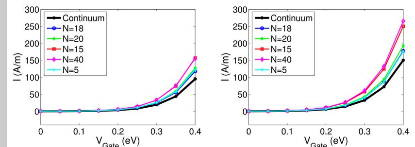
Figure 6: Discrete dopants induced voltage threshold lowering effects
