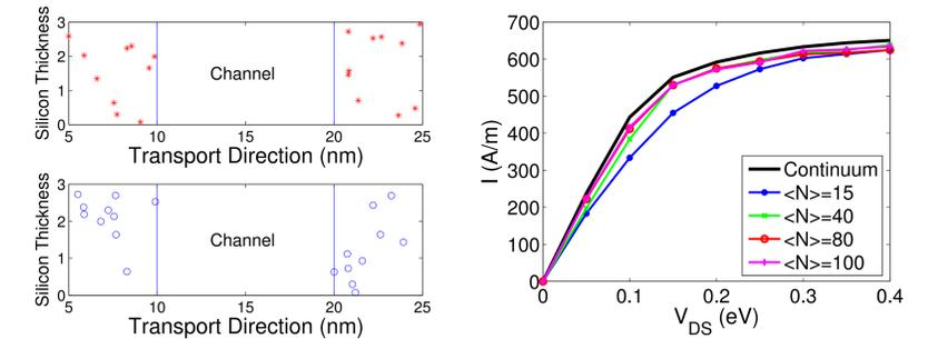
Figure 4: Microscopic dopants distributions make macroscopically identical MOSFET different
