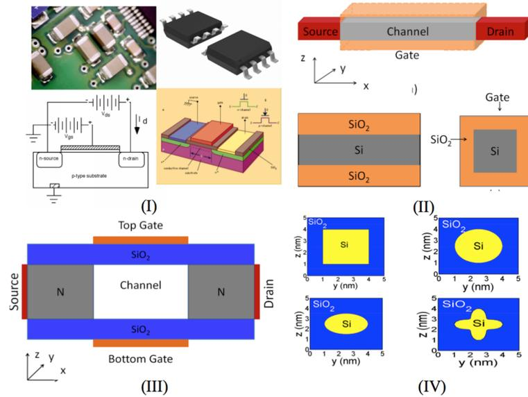
Figure 1: (I) Examples of nano-devices; (II) diagrams of a Four-gate MOSFET; (III) diagram of a DG-MOSFET; (IV) examples of possible material interfaces.
