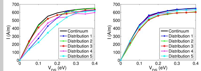
Figure 5: IV curves of nano-MOSFET with individual and continuum dopants
