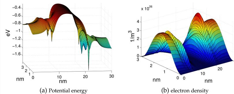
Figure 3: Potential energy and electron density
