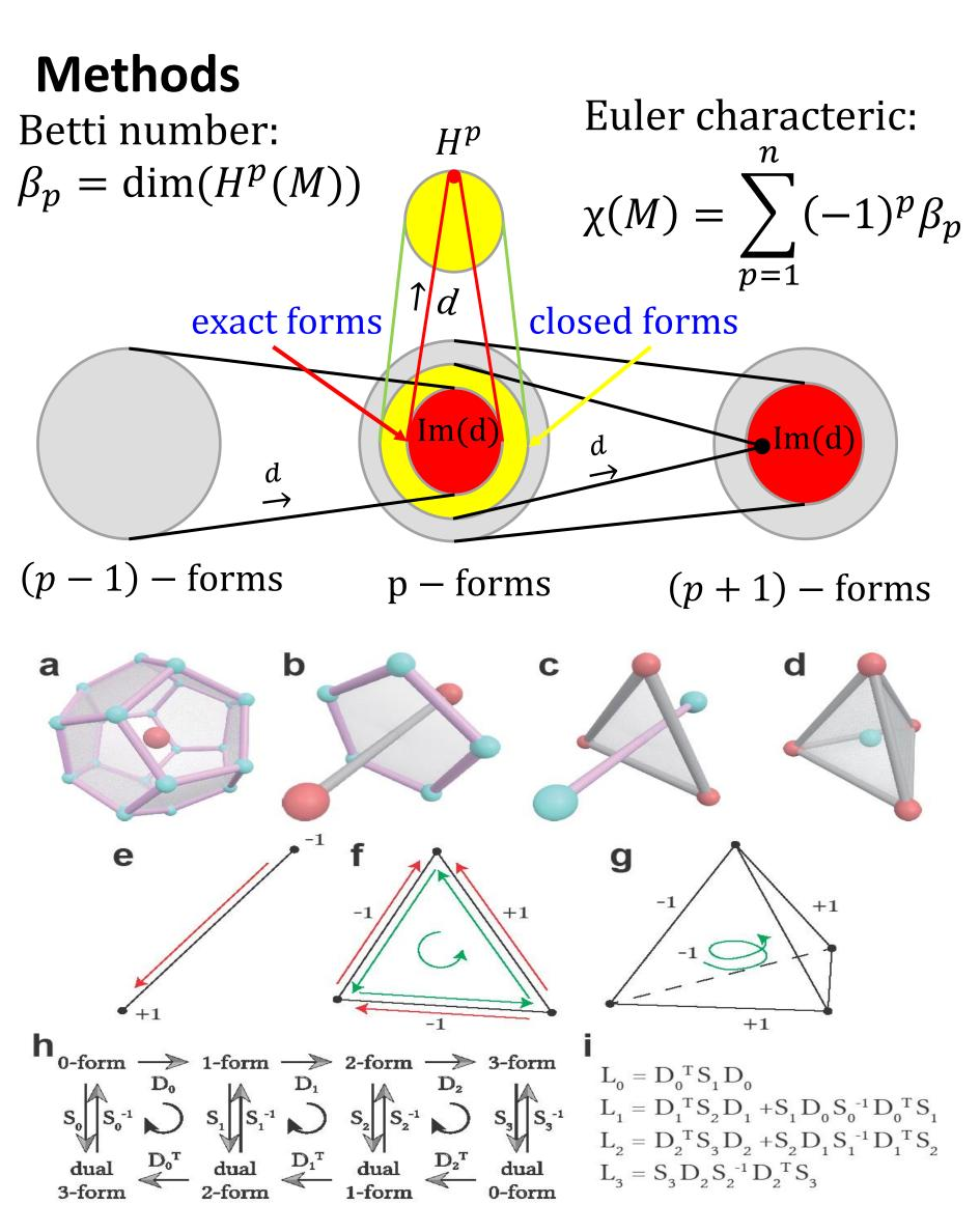
Illustration of *discrete exterior calculus*. **a-d** show the primal and dual elements of the tetrahedral mesh. e-g Illustrate orientation. Pre-assigned orientation is colored in red. Induced orientation by  $\delta$  is colored in green. The vertices are assumed to have positive pre-assigned orientation. **h** describes de Rham's cochain complexes and Hodge duals. i depicts the assembly of four types of Laplace-de Rham operators.
