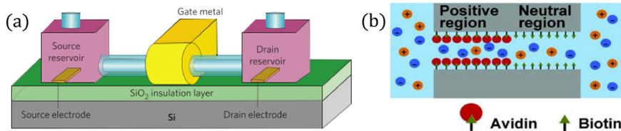
Figure 1: (a) Schematic of a nanofluidic field-effect transistor; (b) Schematic of a nanofluidic diode.
