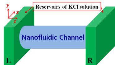
Figure 2: Schematic of a nanofluidic system.
