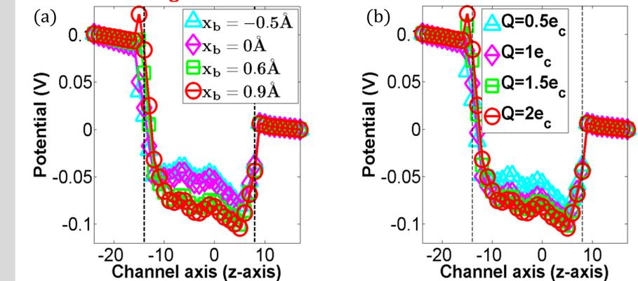
**Figure 2:** Electrostatic potential profiles (a) at different locations of the blocker and (b) at different charges of the blocker.
