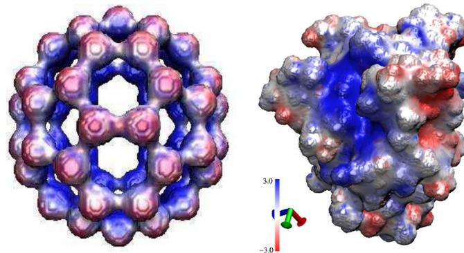
**Figure 3: Electrostatic potential** computed with MMSs generated by Eq. (3). **Left:** with the MMS of  $C_{60}$ ; **Right:** with the MMS of a protein (PDB ID: 1b41). (Bates, Wei and Zhao, J. Comput. Chem. 29, 380 (2008)).
