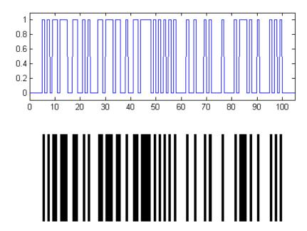
**Figure 2.1.** Samples of the binary bar code function z(t) and the UPC bar code. Note that in UPC bar codes, each bar - black or white - is a multiple of the minimum bar width.
