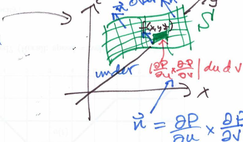
$$\vec{n} = \frac{\partial P}{\partial u} \times \frac{\partial P}{\partial v}$$
