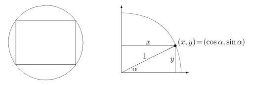
1. Consider the variable  $\alpha$ , the angle between the *x*-axis and the corner point. Then the corner point has coordinates  $(\cos \alpha, \sin \alpha)$ , and we want to maximize the area function  $f(\alpha) = \cos(\alpha) \sin(\alpha)$  on the interval  $0 \le \alpha \le \pi/2$ . (Here  $f(\alpha)$  is  $\frac{1}{4}$  of the beam's cross-section area.)
