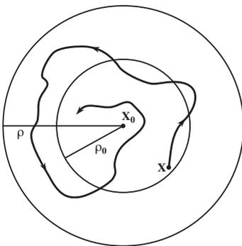
FIGURE 4.1.1. Motion near a stable point  $\mathbf{x}_0$ .
