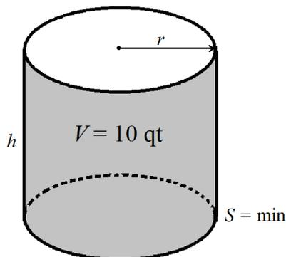
The *target* variable is the surface area  $S$  (square inches), to be minimized. The *controlling* variables are radius  $r$  (inches) and height  $h$  (inches). The constant volume is expressed by the *constrained* variable  $V = 10$  quarts; to make this comparable to the other variables, we must convert to  $V = 577.5$  cubic inches.
