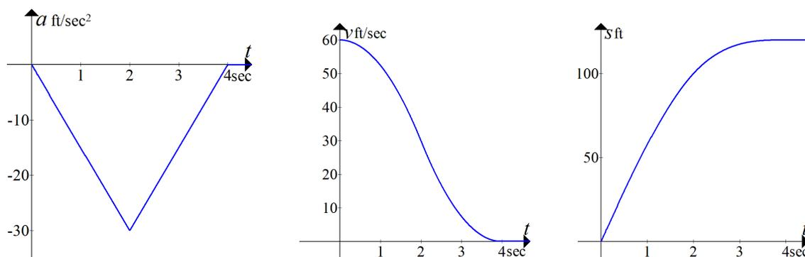
Now the stopping time of 4 sec requires a peak deceleration of  $-30 \text{ ft/sec}^2 \approx 1 \text{ gee}$ , which would send the car skidding helter-skelter. You would need double the time to do this technique safely, starting to brake much earlier.
