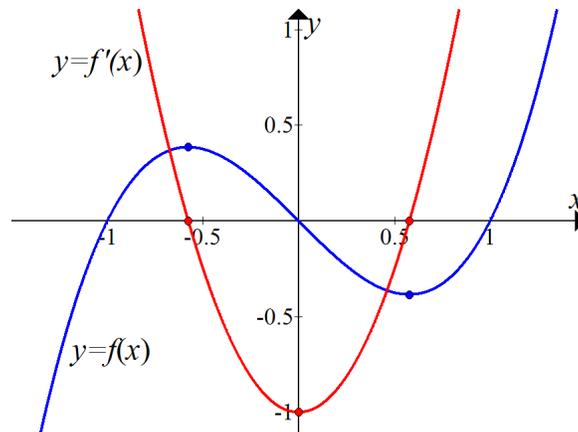
The original graph  $y = f(x)$  has a valley with horizontal tangent at  $x \cong 0.6$ , so the derivative  $f'(0.6) \cong 0$ , and we plot the approximate point  $(0.6, 0)$  on the derivative graph  $y = f'(x)$ ; and similarly the hill on  $y = f(x)$  corresponds to the point  $(-0.6, 0)$  on  $y = f'(x)$ . Between these  $x$ -values, the slope of  $y = f(x)$  is negative, with the slope at  $x = 0$  being about  $-1$ , so  $y = f'(x) < 0$  is below the  $x$ -axis, bottoming out at  $(0, -1)$ .
