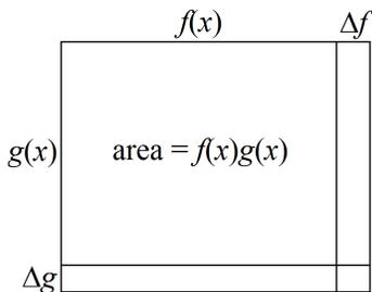
The product  $f(x)g(x)$  is the area, and the derivative  $(f(x)g(x))'$  is the rate of change of area with respect to a change in  $x$ . Suppose small increment  $\Delta x = h$  produces some positive increments  $\Delta f = f(x+h) - f(x)$  and  $\Delta g = g(x+h) - g(x)$  in the sides, so that the increment of area,  $\Delta(f \cdot g) = f(x+h)g(x+h) - f(x)g(x)$ , is the area of the three edge rectangles:<sup>†</sup>
