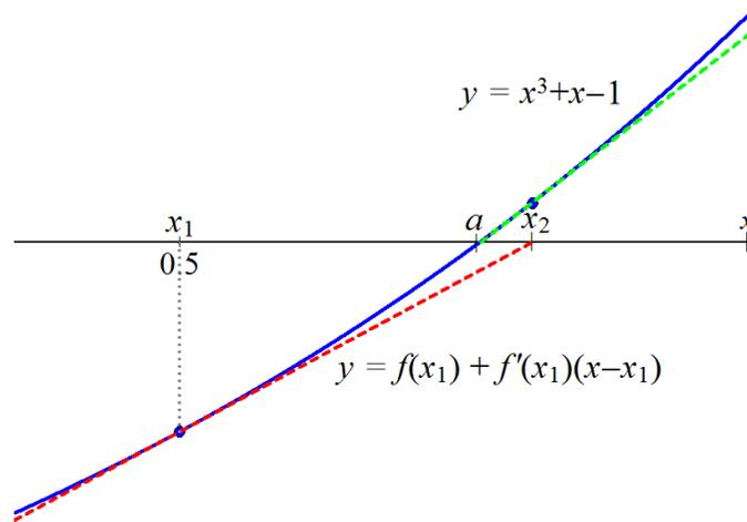
You can see how the tangent line (in red) is very close to the graph near  $x = x_1$ , and fairly close even near the true solution  $x = a$ . We cannot solve for the  $x$ -intercept of  $y = f(x)$ , but we can find the  $x$ -intercept of the line, denoted  $x = x_2$ :
