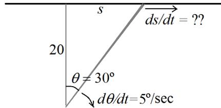
The distance from the wall is the constant 20; the variable quantities are  $\theta$  and  $s$ . The angle  $\theta(t)$  has current value  $\theta(0) = 30^\circ$  and current rate  $\theta'(0) = 5^\circ/\text{sec}$ , and we seek to compute the unknown rate  $s'(0) = \frac{ds}{dt}|_{t=0}$ . From the definition of tangent, we have the equation:  $\tan(\theta) = \frac{s}{20}$ , so we can easily solve for  $s = 20 \tan(\theta)$ . Differentiating (in Leibnitz notation this time):
