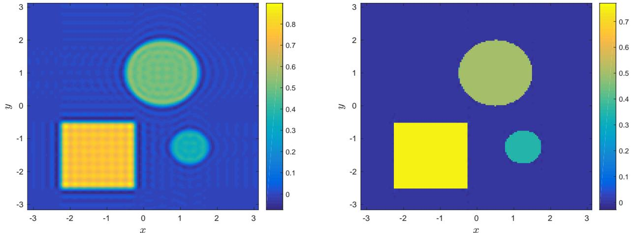
(a) Standard Fourier Reconstruction, PSNR = 26.97 dB.
