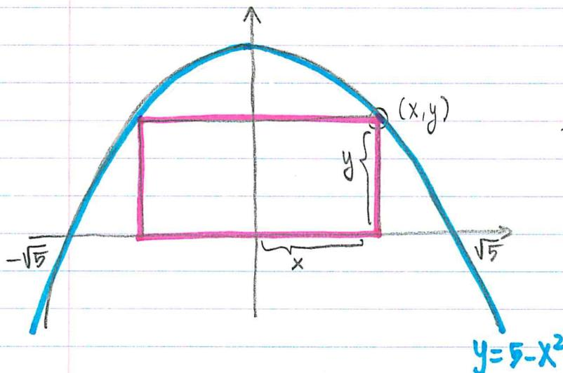
$$\begin{aligned} A &= (2x) \cdot y \\ &= (2x) \cdot (5 - x^2) \\ &= 10x - 2x^3 \end{aligned}$$
