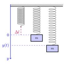
**Theorem 2.6.2.** (Static Equilibrium) A spring with spring constant k, an attached body mass m, at rest with a spring deformation  $\Delta l$ , satisfies
