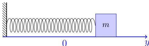
The damping force is proportional to the object's velocity, acting in the opposite direction, and it is given by  $f_d = -dy'$ . Therefore, Newton's equation of motion in this case is
