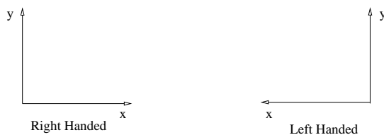
FIGURE 6. Examples of right-handed and left-handed Cartesian coordinate systems, respectively, in two dimensions.
