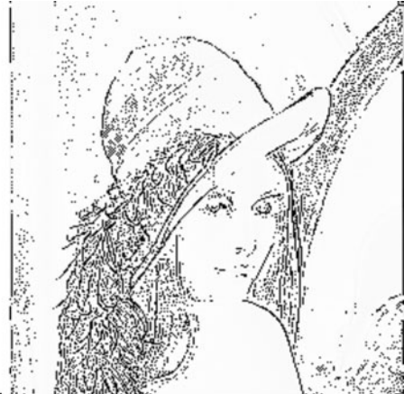
(b) IFD is applied with one mode in total which is essentially a low pass filter mode. Edge is extracted into the first mode.
