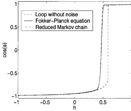
FIG. 13. Simulation of the hysteresis loop with the reduced Markov chain when  $\epsilon=0.01$ .
