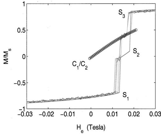
FIG. 2. Hysteresis loops of thin film for different realizations of the noise at  $T=300$  K.
