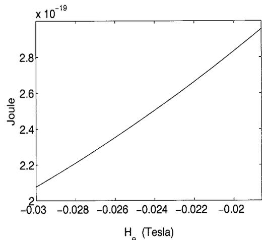
FIG. 18. Energy barriers for the  $S_1 \rightarrow C_A$  switching under different external fields.
