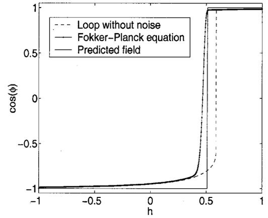
FIG. 12. Predicted switching field for single-domain particle when  $\epsilon = 0.01$ .
