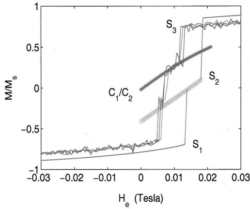
FIG. 5. Hysteresis loops at  $T=1200$  K following the  $S_2 \rightarrow C_1/C_2 \rightarrow S_3$  pathways.
