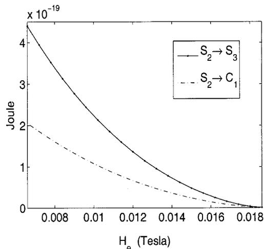
FIG. 16. Energy barriers of  $S_2 \rightarrow S_3$  and  $S_2 \rightarrow C_1$  switchings for different external fields.
