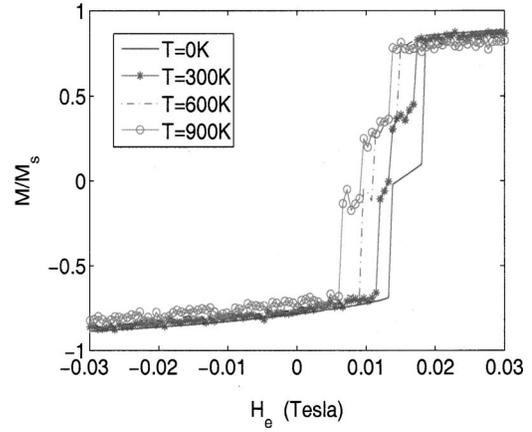
FIG. 4. Hysteresis loops of thin film at different temperatures.
