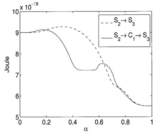
FIG. 17. Energy along the MEPs of  $S_2 \rightarrow S_3$  and  $S_2 \rightarrow C_1 \rightarrow S_3$  switchings when  $H_e=90$  Oe.
