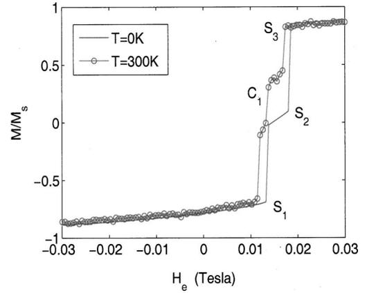
FIG. 1. Hysteresis loops of thin film at  $T=0$  K and  $T=300$  K.
