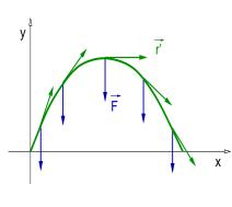
A projectile of mass *m* moving on the surface of Earth.
