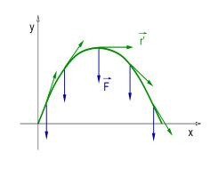
A projectile of mass m moving on the surface of Earth.
