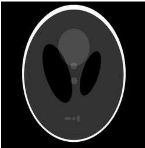
Figure: Same Reconstruction with a further N = 100 Modes estimated using edge information
